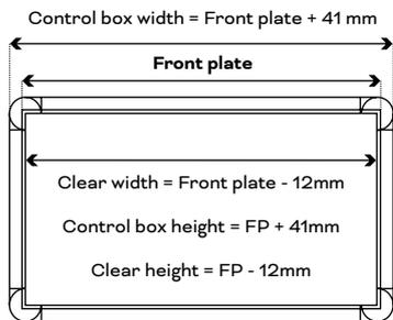
Front plate- / front plate section dimension:
